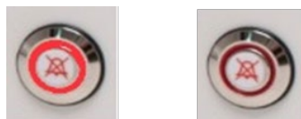
Figure 14.1 Alarm button, which indicates the alarm condition
