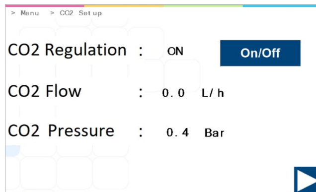
Figure 13.25 CO 2 Setup sub-menu view in the MIRI® TL6 and MIRI® TL12 multiroom IVF incubator
