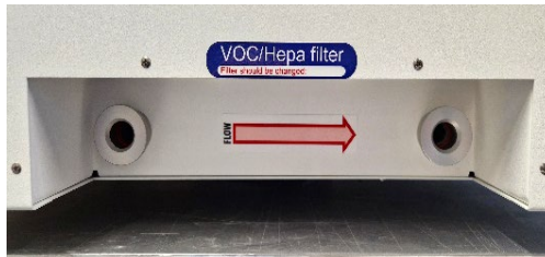
Figure 12.1 The flow arrow on the MIRI® TL6 and MIRI® TL12 multiroom IVF incubators
