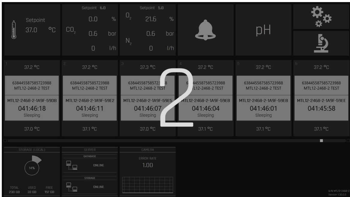
Figure 20.5 Line change indication overlay in the main screen of the MIRI® TL12 multiroom IVF incubator
