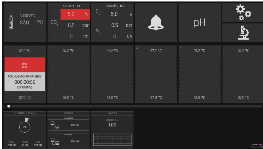
Figure 20.45 CO 2 concentration alarm view
