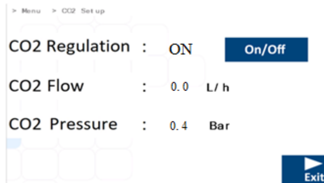
Figure 16.2 CO 2 Setup sub-menu view in the MIRI® TL6 and MIRI® TL12 multiroom IVF incubator
