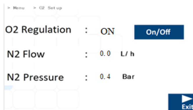
Figure 16.4 O 2 Setup sub-menu view in the MIRI® TL6 and MIRI® TL12 multiroom IVF incubator
