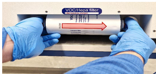
Figure 12.2 VOC/HEPA filter insertion and removal procedure
